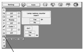
Move the pointer to Lamp counter reset and then press SET button. The message "Lamp replace counter reset?" is displayed.
